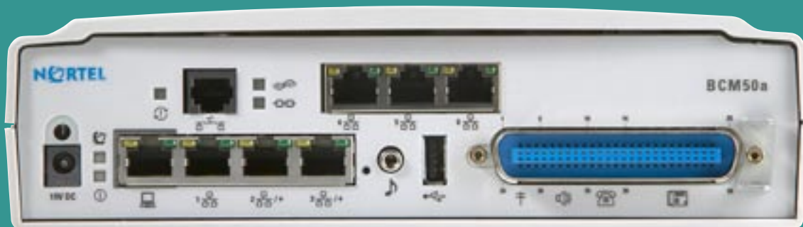
Main unit containing ADSL Router
